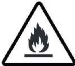
Caution: Risk of fire/ flammable materials (Required for R32/ R290 units only)
